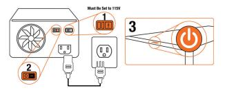
Use the included power cord to connect your power supply unit (PSU) to a wall outlet or surge protector. Turn the power supply switch on before pressing the front power button.
