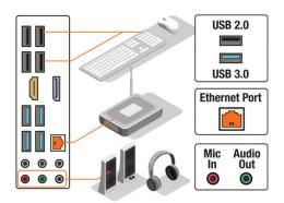
Connect your keyboard, mouse, audio, and network to their matching ports on the motherboard I/O by connection type or color. Any included network adapters or antennas will be in the motherboard box.
