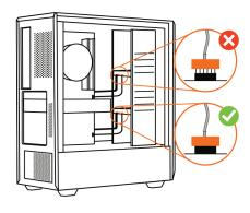
Ensure all component cables are securely connected (some may loosen during shipping). Put the left side panel and screws back on.
