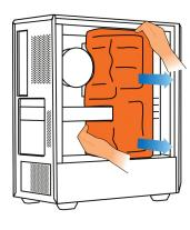
Carefully remove the protective foam.
