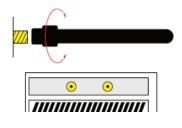
Connect Antennas: The WiFi receiver may come as either 2 separate antennas or a single device with wires that attach to the gold connectors.
