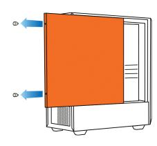
Remove screws from the left side panel. Then remove the panel.
